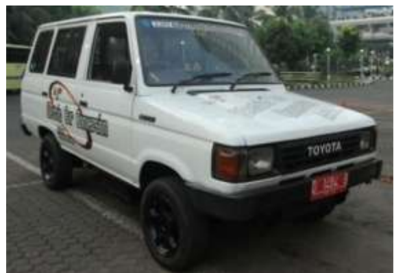
Fig.2 1994 Toyota Kijang Super gasoline-to-electric
